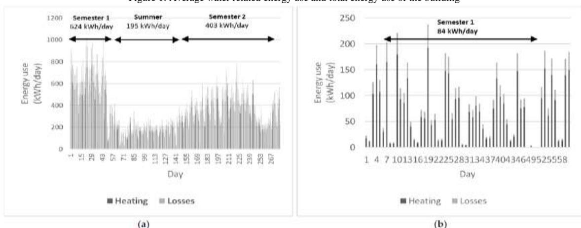
Figure 2. Energy used for water heating in the building (a) before and (b) after the water conservation measures
